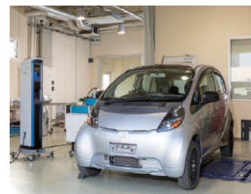
AC普通充電器の互換性評価 Interoperability evaluation of normal AC charger
