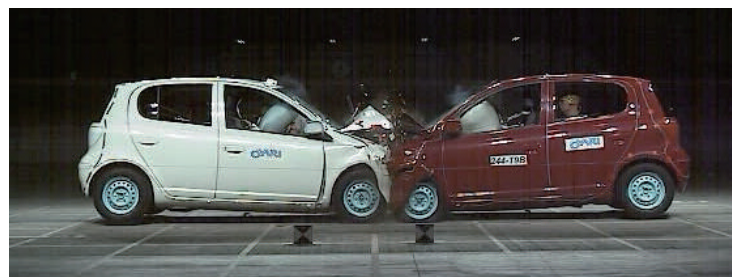
車対車の前面衝突実験 Car-to-car frontal collision test
