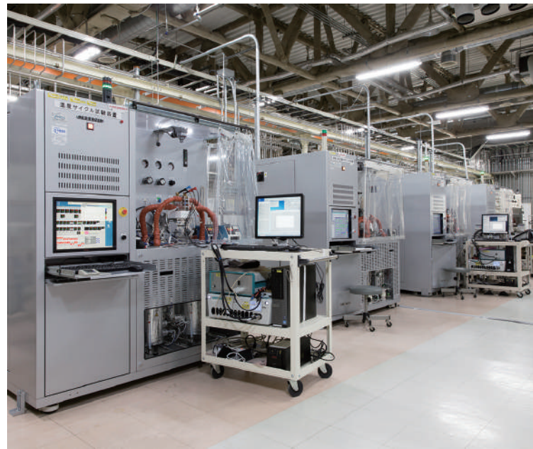
燃料電池単セル性能評価試験装置 Fuel cell single cell performance evaluation test equipment
