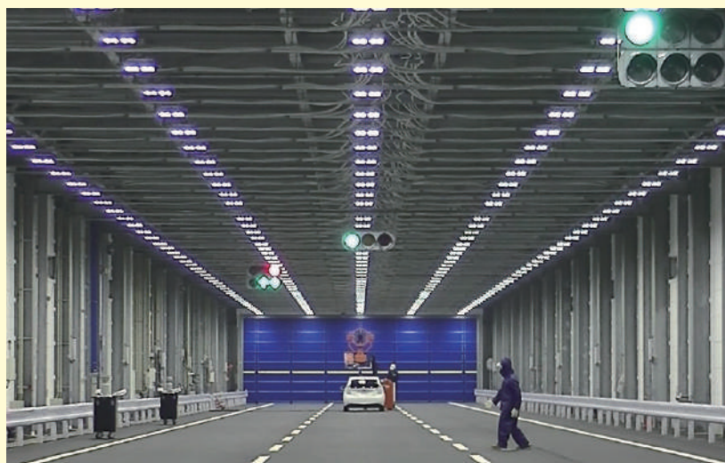
降雨設備での稼動状況 Operational situation of rainfall device
