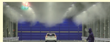
霧発生設備での稼動状況 Operational situation of fog generating device
