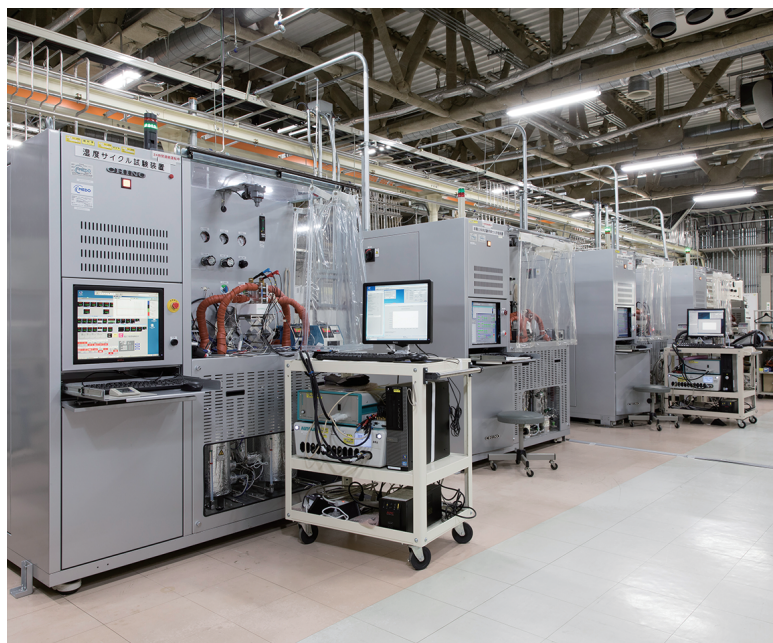
燃料電池単セル性能評価試験装置 Fuel cell single cell performance evaluation test equipment
