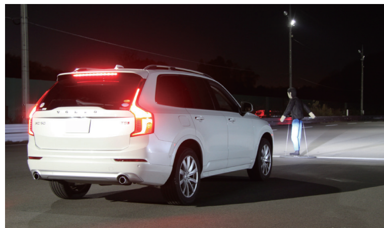
衝突被害軽減ブレーキ(対歩行者[夜間])試験 Evaluation test of autonomous emergency braking (pedestrian [night])
