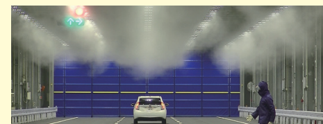
霧発生設備での稼働状況 Operational situation of fog generating device
