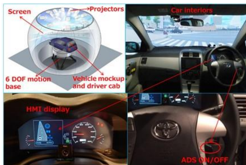
Fig. 1 Top left: structure of the driving simulator. Top right: simulator's interior. Bottom left: HMI screen used to display the status of the system and the surrounding environment. Bottom right: red circled button used to activate and deactivate automated driving mode.
