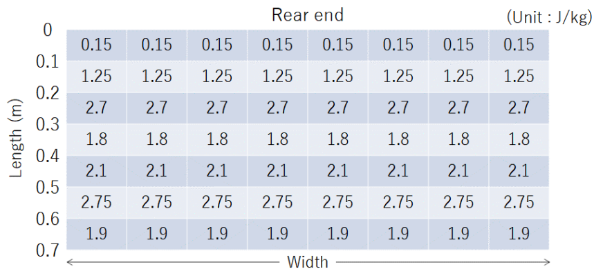
Fig. 11 Rear Crash Energy Absorption Characteristics of Hatchback Sedan Type Hybrid Vehicles
