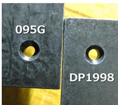
Fig. 3 Difference in Worn Holes
