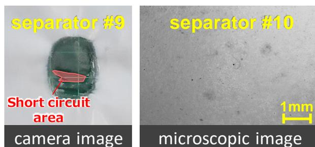
Fig. 5 Results of observation of separators
