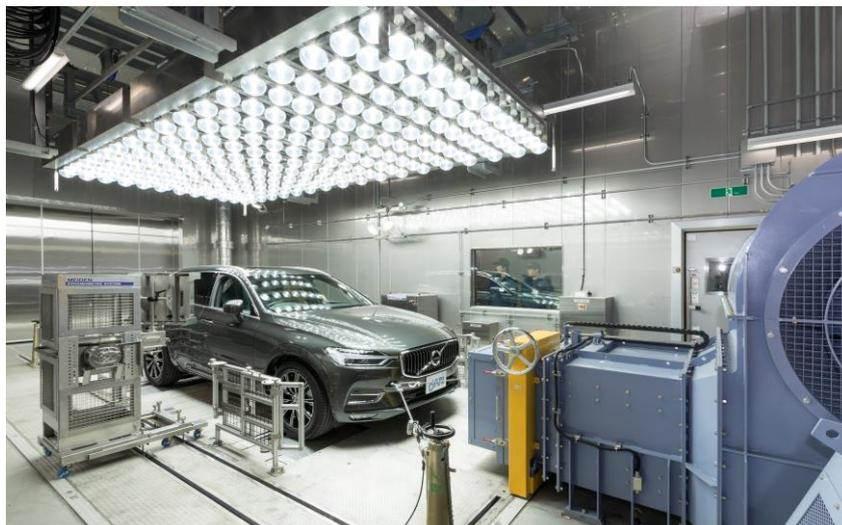
Fig. 5 Appearance of the environmental chassis dynamometer.
