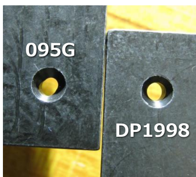
Fig. 3 Difference in Worn Holes
