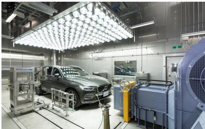
Fig. 5 Appearance of the environmental chassis dynamometer.
