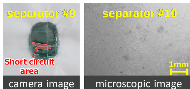
Fig. 5 Results of observation of separators
