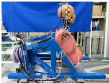
(a) Certification Test without Head restraint
