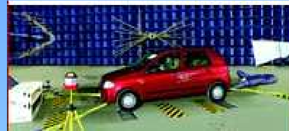
Vehicle EMC Chamber (VRDE)
