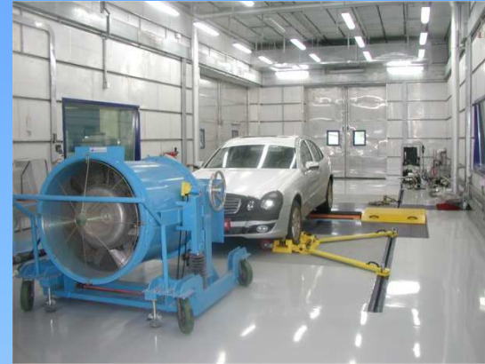
Chassis Dynamometer with Emission Measurement Setup
