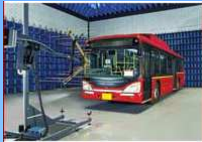
Vehicle EMC Chamber (VRDE)
