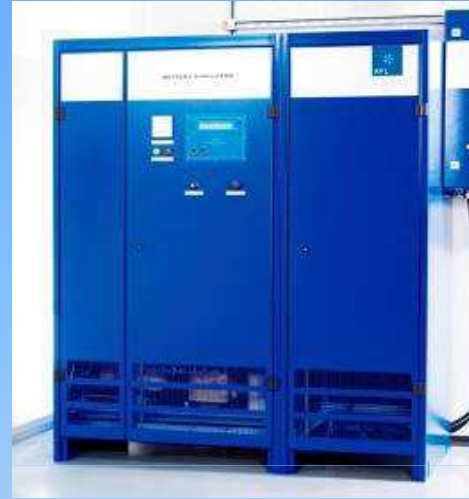
E-Motor Test Bed with Battery Simulator
