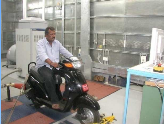
Chassis Dynamometer with Emission Measurement Setup
