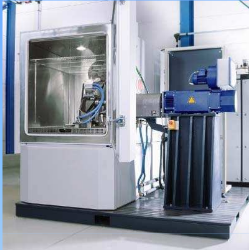
E-Motor Test Bed with Battery Simulator
