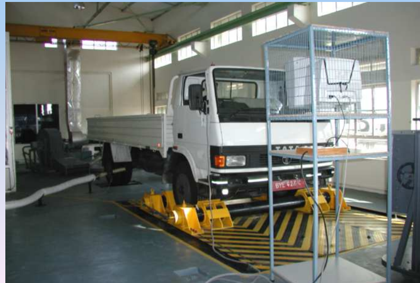
Chassis Dynamometer with Emission Measurement Setup
