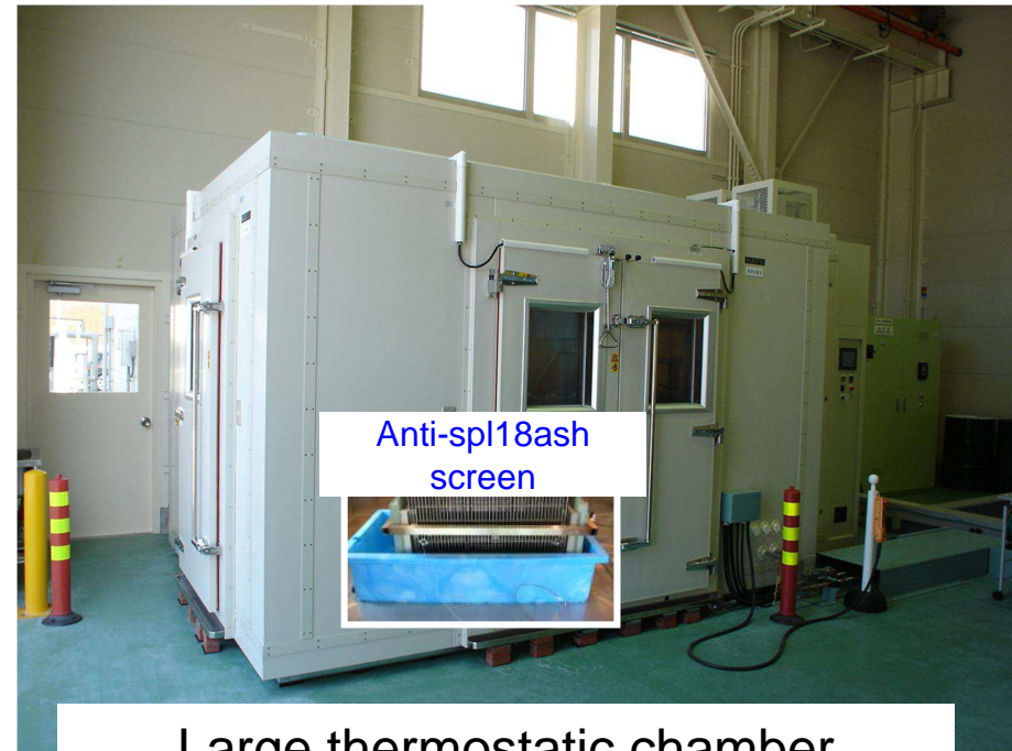
Large thermostatic chamber (-40°C to 150°C, 60% to 98%RH)
