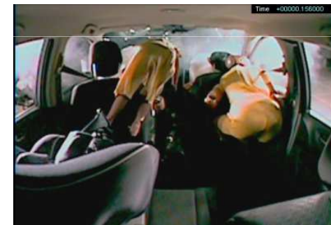
Front-end collision (no belts in rear seats)
