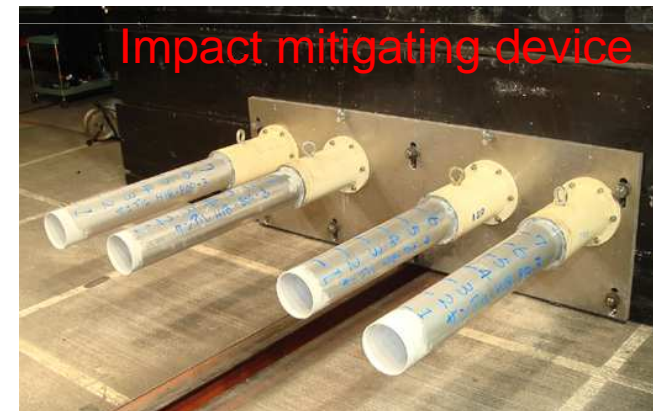
Reproduces impact deceleration by having the vehicle collide with impact mitigating devices (pipes).
