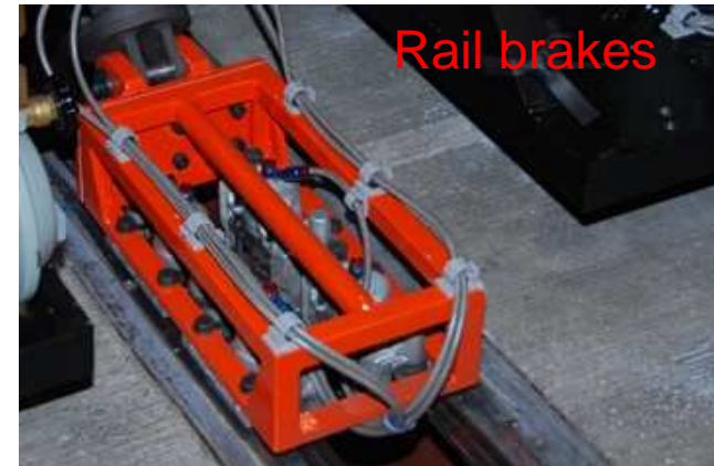
Braking using guide rails
