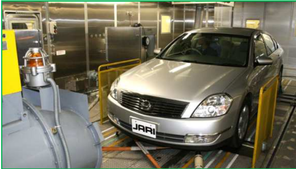
RL-SHED test equipment (with CYD for light duty vehicles)
