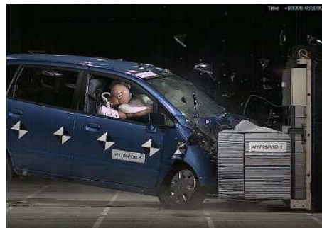
Offset front-end collision
