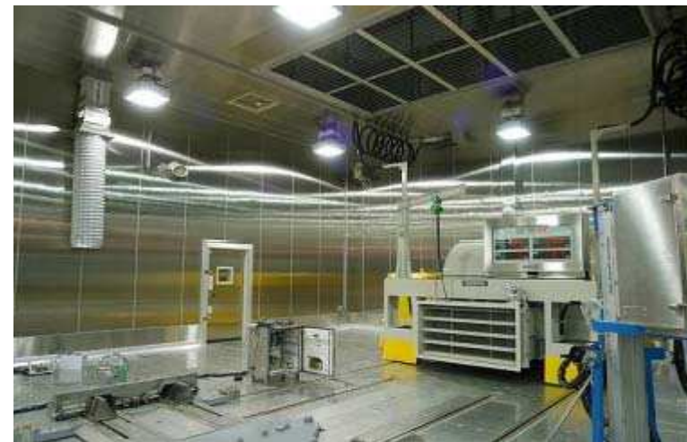
Environmental chassis dynamometer for heavy duty vehicles
